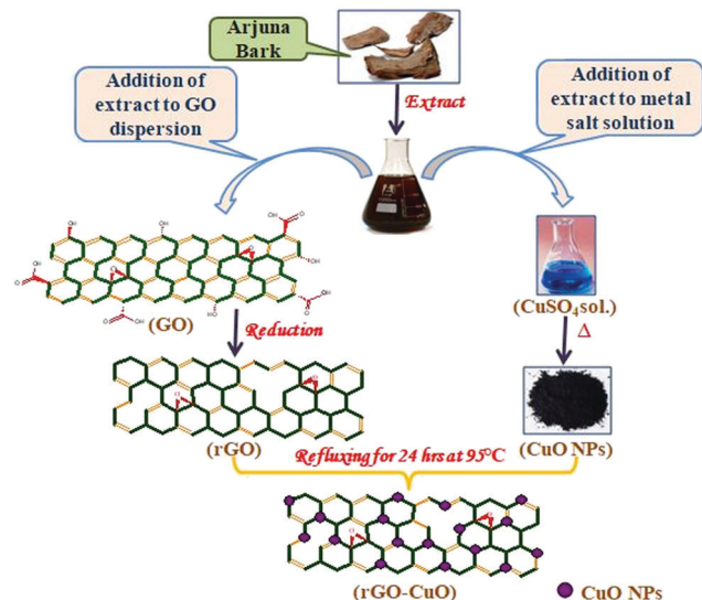
Scheme 1 Schematic for the step-wise synthesis of CuO/rGO nanocomposite.
