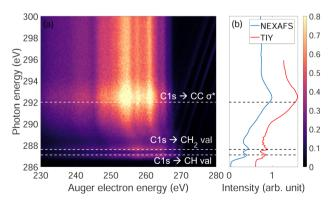
Fig. 3 (a) Two dimensional map of Auger electron kinetic energy as a function of incident photon energy near the C-1s ionization edge of adamantane. (b) Near edge X-ray absorption fine structure (NEXAFS) spectrum and the total ion yield X-ray absorption (TIY) spectrum of adamantane.
