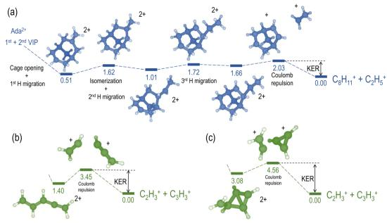
Fig. 8 Potential energy surfaces (DFT-B3LYP/6-31G(d) level) for the channels  $C_2H_5^{+}/C_8H_{11}^{+}$  (a) and  $C_2H_3^{+}/C_3H_3^{+}$  (b) and (c). Relative energies in eV corrected with ZPE and referred to the corresponding exit channel.
