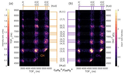
Fig. 10 Zoomed in AEPIPICO of ion pairs recorded in coincidence with CH AES band (a) and CH<sub>2</sub> AES band (b) following ionization of adamantane at  $h\nu$  = 350 eV. The maps have been normalized to maintain the 4:6 (4CH:6CH<sub>2</sub>) ratio that we expect in the adamantane molecule.
