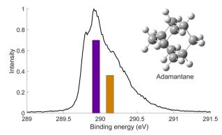
Fig. 1 C-1s XPS spectrum of adamantane recorded at  $h\nu$  = 350 eV. The two bars represent the theoretical contributions of the 2 carbon sites (purple for CH<sub>2</sub> sites and orange for CH sites) and are normalized to 0.7. The strucutre of adamantane is depicted in inset.
