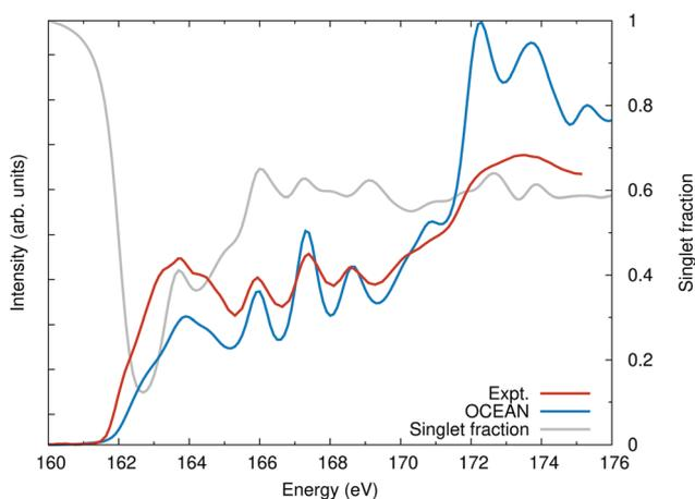
Fig. 1 The calculated sulfur  $L_{2,3}$  edge of CdS compared with experiment.<sup>47</sup> Also shown, the singlet fraction is the ratio of how much of the exciton is due to a spin-up hole and spin-up electron or a spin-down hole and a spin-down electron as a fraction of the total excitonic weight. Without spin-orbit, linearly polarized X-rays will only populate spin-singlet excitons.
