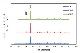
Fig. 4 XRD spectra of KCB, KCB-A and KCB-B.
