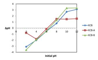
Fig. 1 pHpzc plot for KCB, KCB-A and KCB-B.
