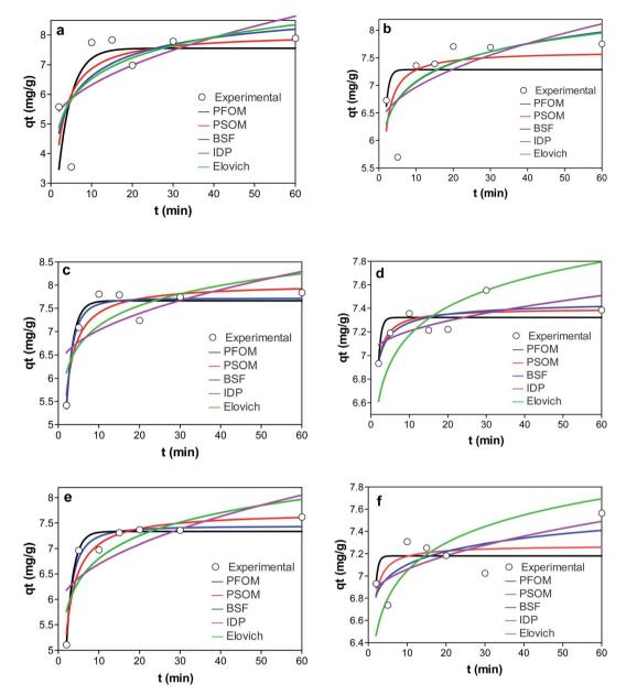
ig. 8 Graphs showing the adsorption kinetics of (a) KCB (b) KCB-A (c) KCB-B on CIP (d) KCB (e) KCB-A and (f) KCB-B on TET.
