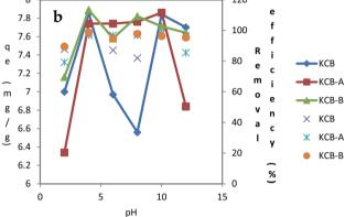
Fig. 5 Effect of pH on the adsorption of (a) TET (b) CIP using KCB, KCB-A and KCB-B (initial concentration =  $40 \text{ mg L}^{-1}$ ; contact time = 60 minutes; adsorbent dosage = 0.05 g; temperature = 303 K).
