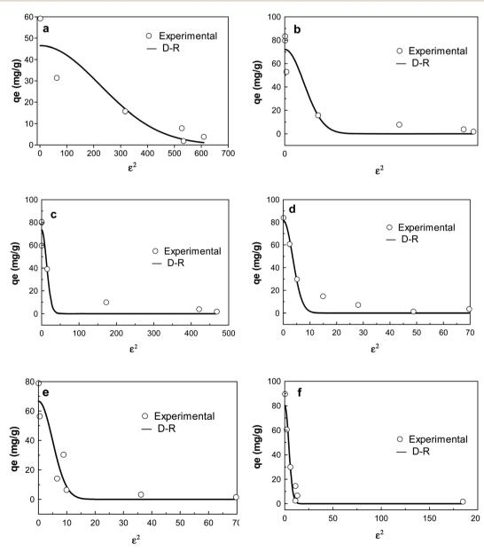
Fig. 7 D-R isotherm plots of adsorption of CIP on (a) KCB (b) KCB-A (c) KCB-B; TET on (d) KCB (e) KCB-A and (f) KCB-B.
