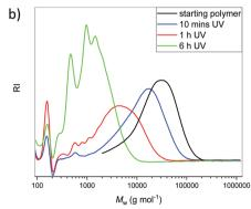
Fig. 5 SEC traces following exposure of poly( $CS_2$ -co-1) ( $M_{n,SEC}$  = 8400,  $D_{\rm M}$  = 1.67) to UV ( $\lambda$  = 365 nm) in the presence of (a) TTMSS (7.5 monomer equiv.) and (b) with no silane present. The reactions were performed at room temperature with  $[poly(CS_2-co-1)]_0 = 0.0267 \text{ mol } L^{-1}$ .
