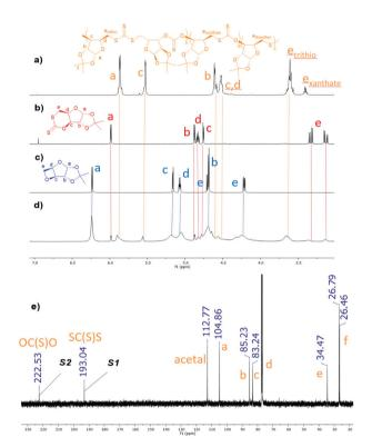
Fig. 1  $^{1}$ H NMR spectra (400 MHz, CDCl<sub>3</sub>) of (a) isolated poly(CS<sub>2</sub>-co-1), (b) 2, (c) 1 and (d) crude poly(CS<sub>2</sub>-co-1) (33% conv of 1); (e)  $^{13}$ C( $^{1}$ H) NMR spectrum (126 MHz, CDCl<sub>3</sub>) of isolated poly(CS<sub>2</sub>-co-1). Reaction performed neat at 80  $^{\circ}$ C with [1]<sub>0</sub>: [CS<sub>2</sub>]<sub>0</sub>: [CrSalen]<sub>0</sub>: [PPNCl]<sub>0</sub> loadings of 100: 200: 1:1 for 4.5 h.
