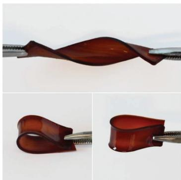
Fig. 3 Images of the cured poly(thioamide-benz-PPEO) film.
