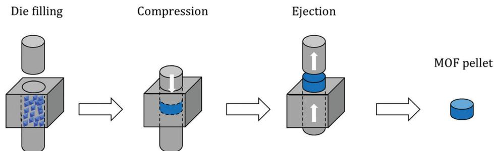
Fig. 1 Schematic representation of the pelletization process applied to polycrystalline MOF powder.
