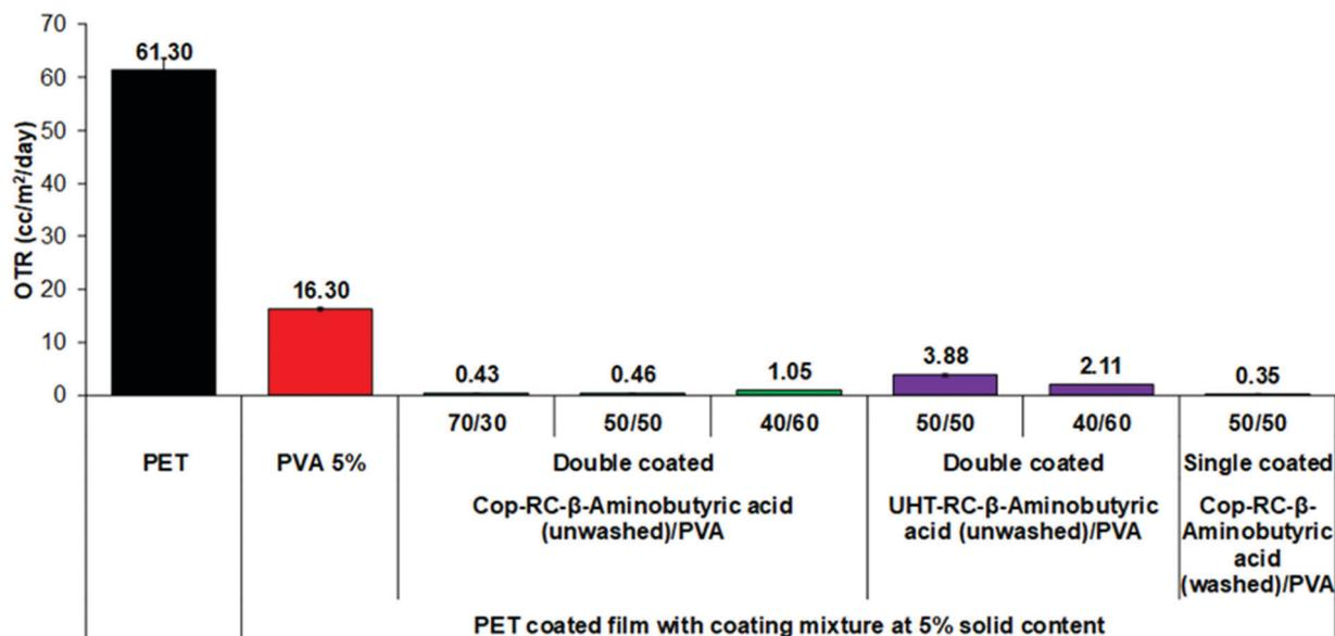
Fig. 3 OTR values of PET, PVA, Cop-RC- $\beta$  aminobutyric acid/PVA/PET film (green) and UHT-RC- $\beta$ -aminobutyric acid/PVA/PET (purple) film with a coating mixture at 5 wt% solid content. Double layer coated film with a coating mixture containing unwashed LDHs/PVA at various ratios. Single layer coated film with a coating mixture containing washed Cop-RC- $\beta$ -aminobutyric acid/PVA at the ratio of 50/50 (blue).
