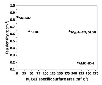
Fig. 3  $\rm N_2$  BET specific surface areas and powder tap densities of different materials. The c-LDH is a conventional water-washed Mg<sub>3</sub>Al-CO<sub>3</sub> LDH. The AMO-LDH is an Mg<sub>3</sub>Al-CO<sub>3</sub> LDH post synthesis dispersed in acetone.<sup>22</sup>
