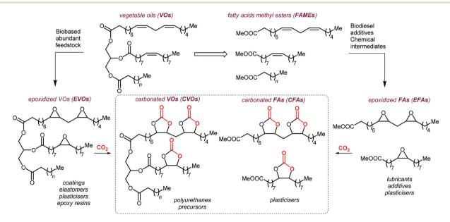
Fig. 5 Products from transesterification and functionalization of vegetables oils depicted as triglycerides of saturated, mono- and poly-unsaturated fatty acids.
