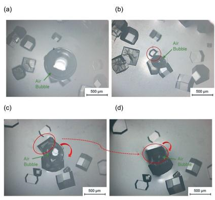
Fig. 3 Microscopic image of a crystal on bubble surface after 6 hours (a) and 55 hours (b) in a hanging drop with condition pH = 4.2, 1.1 M NaCl, and 50 mg mL $^{-1}$  lysozyme and after 77 hours (c) and 140 hours (d) in a different hanging drop with condition pH = 4.2, 1.1 M NaCl, and 70 mg mL<sup>-1</sup> lysozyme.
