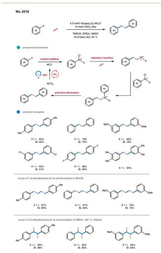
Scheme 19 Ethylene diarylation *via* photoredox and nickel dual catalysis.
