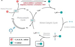
**Scheme 1** (a) Conventional photoredox and nickel dual-catalyzed two-component cross-coupling reactions. (b) Photoredox and nickel dual-catalyzed cascade cross-coupling reactions.
