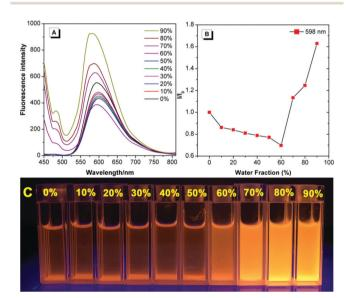
Fig. 2 (A) Fluorescence spectra of TPE-An-Py (1.00  $\times$  10  $^{-4}$  mol L  $^{-1}$ ) in THF/water mixtures with different water fractions ( $\lambda_{ex}$  = 415 nm, slit: 5/5 nm, voltage: 900 V). (B) Plots of  $I/I_0$  values versus the compositions of THF/water mixtures, in which  $I_0$  is the PL intensity in pure THF solution. (C) photographs in THF/water mixtures with different water fractions taken under 365 nm UV irradiation.
