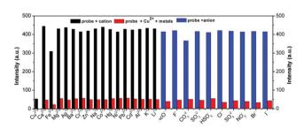
Fig. 5 Bar diagram of the competitive experiments of various metal cations and anions on the fluorescence intensity of the probe/Cu<sup>2+</sup> complex in buffer solution ( $\lambda_{\rm ex}/\lambda_{\rm em}$  = 415/598 nm, slit: 5/5 nm, voltage: 900 V).
