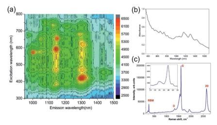
Fig. 3 Spectroscopic analysis of the SWNTs coated plasmonic fibre with *N*-methyl-2-pyrrolidone as the dispersion media (a) photo-luminescence excitation-emission map of excitation wavelength and the observed emission spectra (b) absorption spectra. (c) Raman Spectroscopy at 532 nm excitation.
