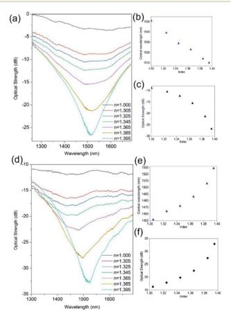
Fig. 4 An example of the variation in refractive index sensitivity of a  $Ge/SiO_2/Pt$  fibre plasmonic device. Before UV processing (a) the transmission spectra as a function of index, (b) central wavelength (c) optical coupling strength. After UV processing (d) the transmission spectra as a function of index, (e) central wavelength (f) optical coupling strength.
