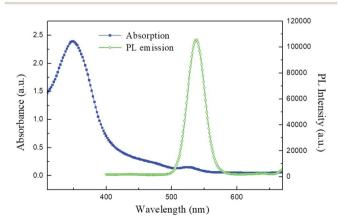
Fig. 3 UV-vis absorption and PL emission spectra of CdSe QDs.
