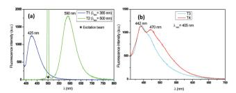
Fluorescence emission spectra of (a) T1 and T2 and (b) T3 and T4
