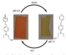
Fig. 12 Schematic of the fabricated textile as a pH sensor/orange-yellow halochromic material.
