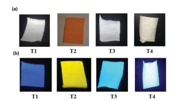
Fig. 6 Sol-gel-treated fabrics (a) upon daylight exposure and (b) upon UV excitation at 365 nm.
