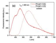
Fig. 10 Emission spectra as a function of pH for the (a) P2, (b) P3, and (c) P4 fluorophores in solution.
