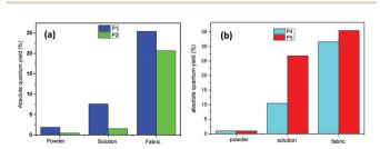
Absolute quantum yields in different types of samples for (a) P1, P2 fluorophores and (b) P3, P4 fluorophores
