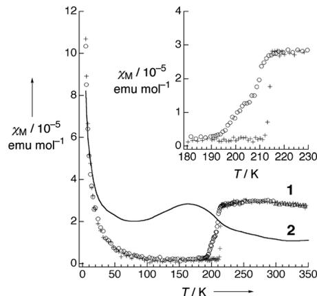
Fig. 6 Temperature dependence of magnetic susceptibility ( $\chi_M$ ) of  $\text{Pt}_2(\text{EtCS}_2)_4\text{I}$  (**2**) and  $\text{Pt}_2(n\text{-BuCS}_2)_4\text{I}$  (**1**;  $\circ$ : 1st cooling,  $+$ : 1st heating,  $\Delta$ : 2nd cooling). Inset shows the phase transition behavior at around 210 K of **1**. Adapted with permission from ref. 33. Copyright 2002 Wiley-VCH.
