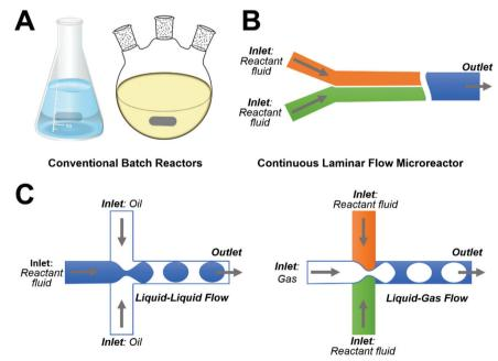
**Discrete segmented Flow Microreactors**
