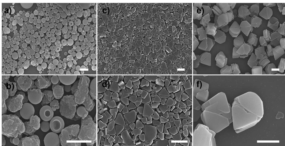
**Fig. 2** SEM images of nanostructures of *R*-SPAN in different  $f_w$ : (a and b) 50%, (c and d) 85% and (e and f) 90%, respectively. ( $[R\text{-SPAN}] = 1.5$  mM, scale bar 1  $\mu$ m). Upon increasing the fraction of water, the morphologies transformed from 0D nanospheres with a rough surface or with a hole to 2D and finally to 3D layered nanoflakes.
