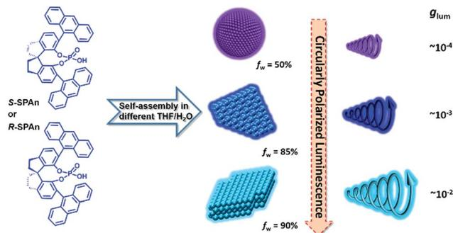
**Scheme 1** Self-assembly of chiral molecules into different nanostructures in mixed THF/H<sub>2</sub>O with different volume ratios. Upon increasing the volume fraction of water, assembled structures of nanoparticles, and 2D and 3D nanoflakes were obtained. The CPL of the aggregates obtained in various water fractions was gradually amplified and the  $g_{\text{lum}}$  value of 3D nanoflakes finally increased by two orders of magnitude in comparison with the monomeric molecules.
