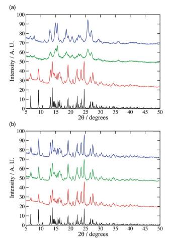
Fig. 1 PXRD patterns for the aspirin:meloxicam co-crystal obtained from experiments at 25 Hz (red), 15 Hz (green) and 10 Hz (blue) employing both (a) neat grinding conditions and (b) LAG conditions with 0:05 mol equiv. of CHCl<sub>3</sub>. The simulated single crystal X-ray diffraction pattern (black) for the co-crystal is shown in both plots (CSD code: ARIFOX).
