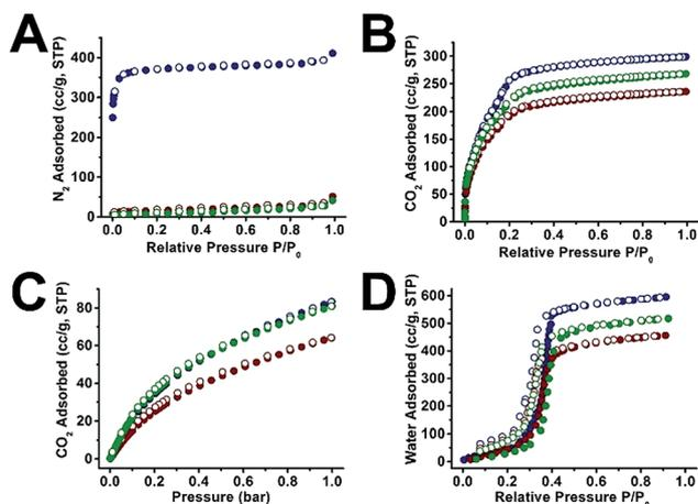
Fig. 4 N<sub>2</sub> sorption isotherms at 77 K (A), CO<sub>2</sub> sorption isotherms at 195 K (B) and 273 K (C), and water vapor sorption isotherms at 298 K (D) of UiO-66 (navy), UiO-66@xPS (red) and UiO-66@xPBA (green). UiO-66@xPS and UiO-66@xPBA isotherms were normalized by subtracting the mass of the polymer (Table S5†).
