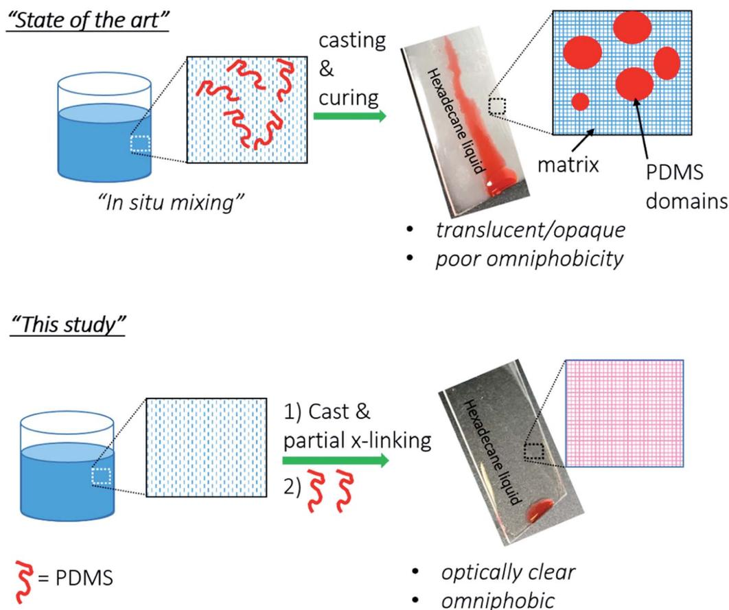
**Scheme 1** Schematic illustrations of our novel top-layer approach (“This study”) versus the conventional approaches (“State of the art”) to fabricate omniphobic surfaces.
