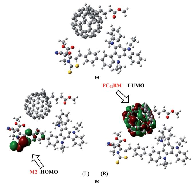
Fig. 11 (a) Optimized geometry of  $M2:PC_{61}BM$  complex at B3LYP/6-311G(d,p) level of theory. (b) Charge transfer between donor M2 (HOMO) on left (L) side and polymer acceptor  $PC_{61}BM$  (LUMO) on right (R) side at B3LYP/6-311G(d,p) level of theory.
