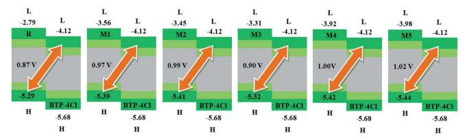
Fig. 8 The value of open circuit voltage ( $V_{oc}$ ) of reference R and designed molecules M1-M5 with respect to the acceptor moiety BTP-4Cl.
