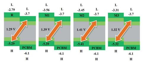
Fig. 7 The value of open circuit voltage (Voc) of reference R and designed molecules M1-M3 with respect to the acceptor moiety PC61BM.
