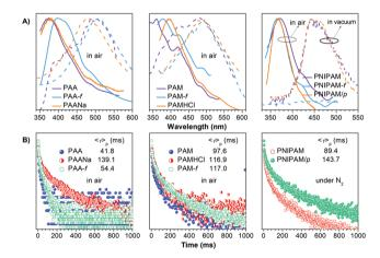
Fig. 4 (A) Emission spectra with  $t_d$  of 0 (solid line) and 0.1 ms (dash line) and (B) RTP decay curves of different films (f) and powders in air, under nitrogen, or in vacuum. Detailed  $\lambda_{ex}$ s for the emission measurement and monitored wavelengths for the lifetime test are listed in Tables S1 and S2 (ESI†).
