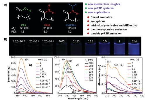
Fig. 1 (A) Structures, M<sub>w</sub>, PDI and features of PAA, PAM and PNIPAM. (B) Different PNIPAM/DMF solutions taken under 365 nm UV light. PL spectra of (C) different PNIPAM/DMF solutions ( $\lambda_{ex}$  = 310 nm) and (D) 2 M solution with different  $\lambda_{ex}$ s. (E) Absorption spectra of different PNIPAM/DMF solutions.
