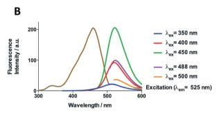
Fig. 1 (A) TEM image of FCD-3 and distribution of diameters between 1.8 and 3 nm. (B) Fluorescence emission and excitation spectra showing that fluorescence emission is excitation independent.
