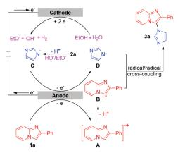
Proposed mechanism of the intermolecular oxidative C-H/ N-H cross-coupling reaction.
