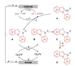
Scheme 4 Proposed mechanism of the intramolecular oxidative C-H/ N-H cross-coupling reaction.
