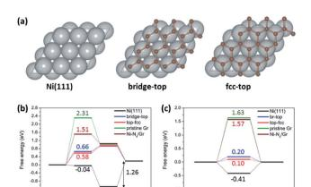
Fig. 5 (a) Calculation models for Ni(111) and two graphene structures (bridge-top and fcc-top) for Gr/Ni(111). The free energy diagrams for (b) electrochemical  $CO_2$  reduction to CO and (c) the HER on Ni(111),  $CO_2$  Gr/Ni(111), pristine graphene and  $CO_3$  Ni- $CO_4$  Ni-
