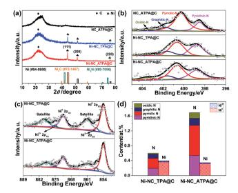
Fig. 1 (a) XRD patterns and (b) N 1s XPS spectra of N doped carbon without Ni (NC\_ATPA@C), Ni-NC\_TPA@C, and Ni-NC\_ATPA@C. (c) Ni 2p XPS spectra. (d) Atomic contents of N species including pyridinic N, pyrrolic N, graphitic N, and oxidic N, and Ni species including Ni<sup>0</sup> and Ni<sup>2+</sup> of Ni-NC\_TPA@C and Ni-NC\_ATPA@C based on XPS
