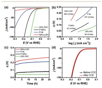
Fig. 3 (a) IR-corrected linear sweep voltammetry (LSV) curves, with a scan rate of 5 mV s $^{-1}$ . (b) Tafel plots and (c) current density traces of CCE at 10 mA cm $^{-2}$  for HER in 1.0 M KOH. (d) LSV curves for P-NiFe before (black line) and after (red line) CCE for HER at 10 mA cm $^{-2}$  for 25 h. Catalysts: P-NiFe (black), NiFe-LDH (red), P-Ni (blue) and 20% Pt/C (green).
