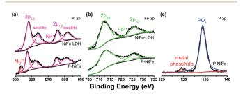
Fig. 1 The XPS patterns of as-prepared  $Ni_2P@FePO_x$  sample, showing the signals of (a) Ni 2p, (b) Fe 2p and (c) P 2p.
