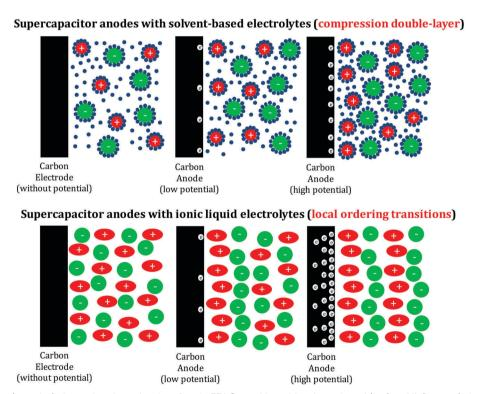
Fig. 3 Schematic of the (negative) electrode-electrolyte interface in EDLCs working with solvent-based (top) and IL (bottom) electrolytes. While energy storage in the former is based on double-layer compression and thus requires transport of electrolyte ions, local ordering transitions (i.e. changes in the ion coordination numbers) are responsible for the energy storage in the absence of a solvent.
