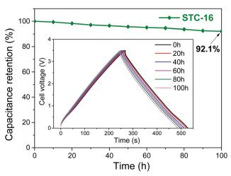
Fig. 4 Floating stability of STC-16 at a specific current of 1 A  $g^{-1}$  for 100 h of floating at 3.5 V. The inset shows the charge/discharge profiles every 20 h. Figures reproduced with permission from ref. 21
