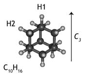
Fig. 1 Structure of the adamantane molecule  $C_{10}H_{16}$ . The arrow shows the  $C_3$  rotation axis along which the adamantyl cation deforms, due to Jahn–Teller effect. H1 and H2 identify two non-equivalent H atoms in the cations.
