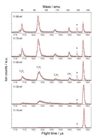
**Fig. 3** Threshold ionisation mass spectra of adamantane at photon energies of 11.10, 11.30, 11.50, 11.70 and 11.90 eV (open circles) plotted together with model fits to the data (red lines). The star (\*) marks a contamination that is present in the system, but does not interfere with the measurements. The peaks are labeled according to the correspondent loss channel. Due to insufficient mass resolution, H-loss peak is unresolved, see Section 3.1.3 for details.
