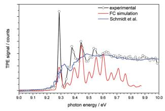
Fig. 2 Threshold photoelectron spectrum of adamantane plotted together with a simulated spectrum (red line) and the conventional photoelectron spectrum of Schmidt et al.<sup>32</sup> (blue line).
