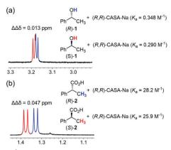
Fig. 2 Partial <sup>1</sup>H NMR spectra and measured binding constants for chiral solvation of (a) 1-phenylethanol (1) and (b) 2-phenylpropionic acid (2) with (R,R)-CASA-Na at 25 °C in CD<sub>3</sub>CN.
