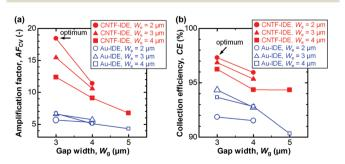
Fig. 4 (a) The amplification factor (AF $_{CV}$ ) and (b) the collection efficiency (CE) with CV with different electrode structures. The data with the optimum electrode structure ( $W_e = 2 \mu m$  and  $W_q = 3 \mu m$ ) are shown
