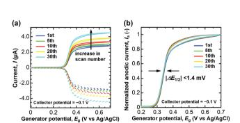
Fig. 8 (a)  $I_a$  (solid line) and  $I_c$  (dashed line) in 30 times repeated dual-mode CV of DA (100  $\mu$ M) in PBS (pH 7.4) with the CNTF-IDE ( $W_e=2~\mu$ m and  $W_a=3~\mu$ m) at  $v=10~mV~s^{-1}$ . (b) Normalized  $I_a$  by that at 0.7 V.
