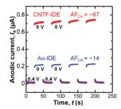
Fig. 5 Anodic current  $(I_a)$  at the generator in the dual-mode CA with the Au-IDE or the CNTF-IDE ( $W_{\rm e}=2~\mu{\rm m}$  and  $W_{\rm g}=3~\mu{\rm m}$ ). The generator potential was fixed at 0.4 V, and the collector potential was stepped as shown in the graph (0 V and 0.4 V). The potential is the value against the Ag/AgCl reference electrode.
