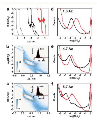
Fig. 2 (a) Typical individual traces for single-molecule conductance measurement of 1,3Az without (black) and with (red) TFA, and the blank (gray). 2D conductance histograms and stretched distance distributions (inset) for 1,3Az (b) without and (c) with TFA. (d-f) Conductance histograms of 1,3Az, 4,7Az and 5,7Az without (black) and with (red) TFA.
