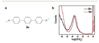
Fig. 3 (a) Molecular structure of molecule **Be** for the control experiment. (b) Conductance histograms of molecule **Be** with (red) and without (black) TFA.
