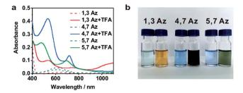
Fig. 1 (a) UV-vis spectra of 1,3Az, 4,7Az, and 5,7Az with/without TFA. (b) Color changes of Az solutions before (left) and after (right) adding TFA.
