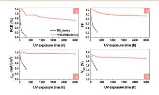
Fig. 5 The evolution of solar cell parameters (normalized (a):  $V_{\rm OC}$ , (b):  $J_{\rm SC}$ , (c): FF, (d): PCE) as a function of testing time under UV illumination for the PFN-2TNDI- and TiO<sub>2</sub>-based perovskite solar cells. The devices were stored under exposure to UV in a N<sub>2</sub>-filled glove-box during testing.
