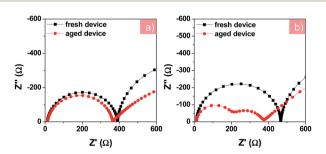
Fig. 6 Nyquist plots of fresh and aged devices based on PFN-2TNDI (a) and  $TiO_2$  (b) under illumination at a bias of -0.7 V. The aged devices were under exposure to constant UV light in an argon-filled glove box for 200 h before testing
