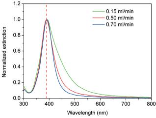
Fig. 16 Normalised UV-vis extinction spectra of Ag nanoparticles synthesized in helical tubular microreactors with different total flow rates. Conditions: reactor length: 130 cm, helix diameter: 14 mm, pitch:  $1/\pi$ mm, AgNO<sub>3</sub>/NaBH<sub>4</sub> molar ratio of 1:6 at 60 °C.
