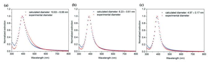
Fig. 17 Fitting of the experimental UV-vis spectra of silver nanoparticles synthesized in helical reactors with varying total flow rates of (a) 0.15 ml  $min^{-1}$ , (b) 0.5 ml  $min^{-1}$  and (c) 0.7 ml  $min^{-1}$ , a length of 130 cm, a helix diameter of 14 mm, and a helix diameter of  $1/\pi$  mm with an AgNO<sub>3</sub>/NaBH<sub>4</sub> molar ratio of 1:6 using the Mie model.
