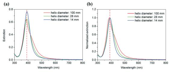
Fig. 7 UV-vis extinction spectra (a) and normalized extinction spectra (b) for AgNPs synthesized in helical tubular microreactors with different helix diameters. Conditions: helix length: 130 cm, helix pitch:  $1/\pi$  mm, and total flow rate: 0.7 mL min<sup>-1</sup> with an AgNO<sub>3</sub>/NaBH<sub>4</sub> molar ratio of 1:6.
