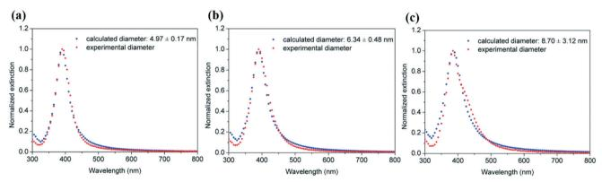
Fig. 8 Fitting of the experimental UV-vis spectra of AgNPs synthesized in helical tubular microreactors with varying helix diameters of (a) 14 mm, (b) 28 mm and (c) 100 mm using the Mie model. Conditions: reactor length: 130 cm, helix pitch:  $1/\pi$  mm and total flow rate: 0.7 mL min<sup>-1</sup> with an AgNO<sub>3</sub>/NaBH<sub>4</sub> molar ratio of 1:6.
