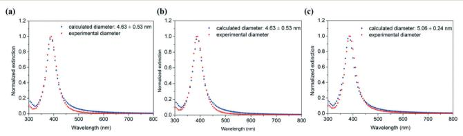
Fig. 14 Comparison of experimental UV-vis spectra of Ag NPs synthesized in helical tubular microreactors with varying helix pitch values of (a)  $1/\pi$  mm, (b)  $2.5/\pi$  mm and (c)  $5/\pi$  mm, a length of 60 cm, a helix diameter of 14 mm and a total flow rate of 0.7 mL min<sup>-1</sup> with an AgNO<sub>3</sub>/NaBH<sub>4</sub> molar ratio of 1:6 and the predicted ones using the Mie model.
