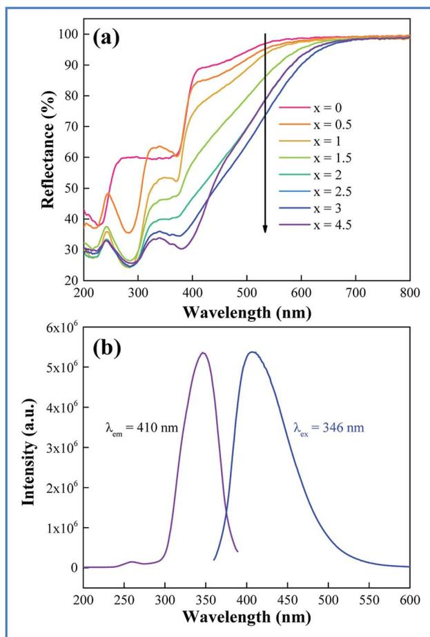
Fig. 2 (a) UV-vis diffuse reflection spectra of the as-synthesized phosphors CAZO: $x\%$  Bi<sup>3+</sup> with different concentrations,  $x$ , of Bi<sup>3+</sup> ( $x = 0, 0.5, 1, 1.5, 2, 2.5, 3$  or  $4.5$ ). (b) Excitation ( $\lambda_{em} = 410$  nm) and emission ( $\lambda_{ex} = 346$  nm) spectra of a typical sample of CAZO:1% Bi<sup>3+</sup>.
