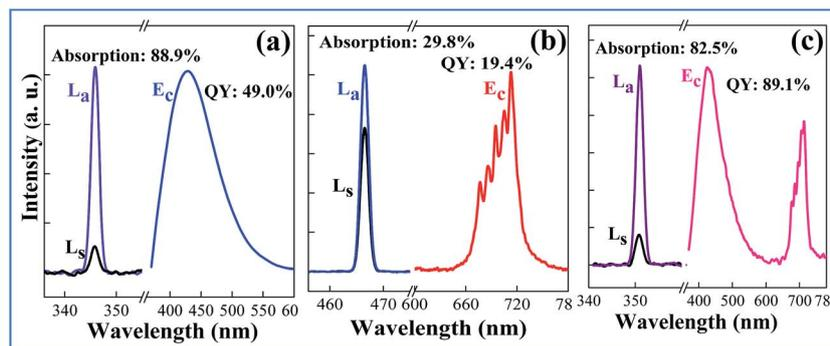
Fig. 7 The excitation lines and emission spectra of the as-prepared samples (a) CAZO:0.5% Bi<sup>3+</sup>, (b) CAZO:0.5% Mn<sup>4+</sup>, and (c) CAZO:1% Bi<sup>3+</sup>, 0.5% Mn<sup>4+</sup> for measurement of the quantum yield using an integrating sphere.
