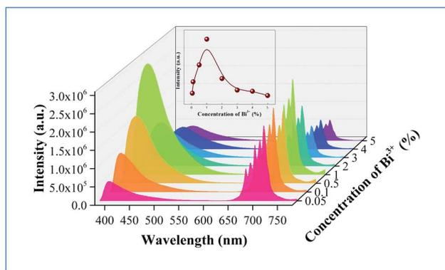
Fig. 8 Emission ( $\lambda_{\text{ex}} = 351 \text{ nm}$ ) spectra of typical samples of CAZO: $x\%$  Bi<sup>3+</sup>, 0.5% Mn<sup>4+</sup> ( $x = 0.05, 0.1, 0.5, 1, 2, 3, 4$  or  $5$ ). Insert: the total luminescence intensities from both Bi<sup>3+</sup> and Mn<sup>4+</sup> varied with the concentration of Bi<sup>3+</sup> ions.
