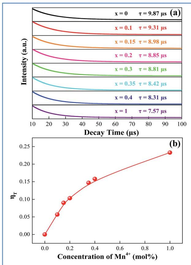
Fig. 5 (a) Decay curves (monitored at 410 nm and excited at 346 nm) of  $\text{Bi}^{3+}$  in the CAZO:0.5%  $\text{Bi}^{3+}$ ,  $x\%$   $\text{Mn}^{4+}$  ( $x = 0.05\text{--}0.5$ ) phosphors. (b) The efficiency of energy transfer from  $\text{Bi}^{3+}$  to  $\text{Mn}^{4+}$  as a function of  $\text{Mn}^{4+}$  concentration.
