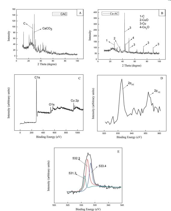
Fig. 4 XRD spectra of CAC (A), Cu-AC (B), the wide scan XPS spectrum of the Cu-AC (C), XPS of Cu-AC (D), and the peaks O 1s of Cu-AC (E).
