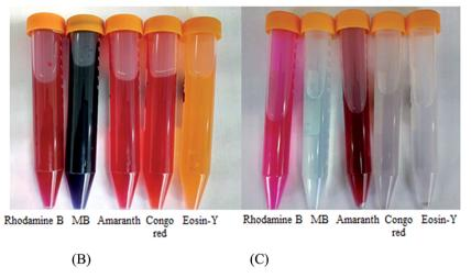
Fig. 8 The adsorption performance of Cu-AC for five dyes: (A) picture of Cu-AC before, (B) and after, (C) adsorbed five dyes.
