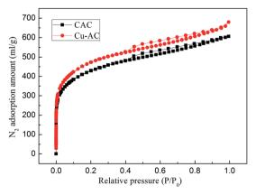
Fig. 2 N<sub>2</sub> adsorption-desorption isotherms of the CAC and Cu-AC.
