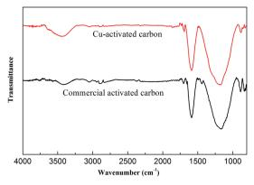
Fig. 6 Fourier transform infrared spectroscopy (FTIR) of commercial activated carbon and Cu-activated carbon.
