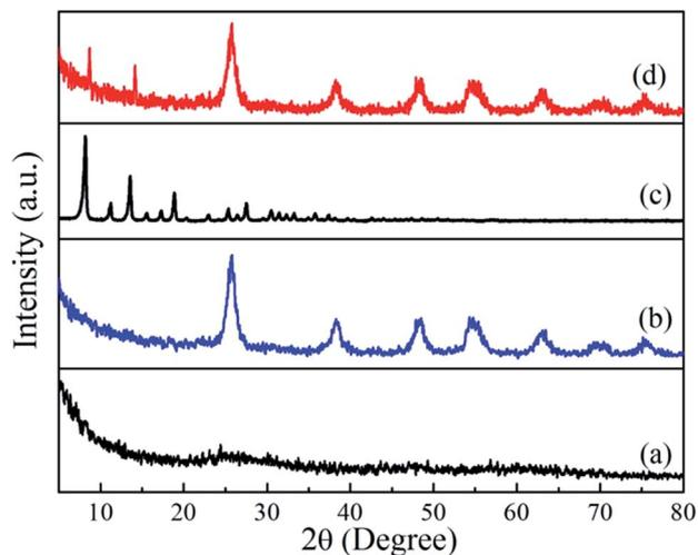
Fig. 1 Powder X-ray diffraction patterns of (a) TiO<sub>2</sub> colloids, (b) TiO<sub>2</sub> beads, (c) pure ZIF-8, and (d) TiO<sub>2</sub>/ZIF-8 spheres.
