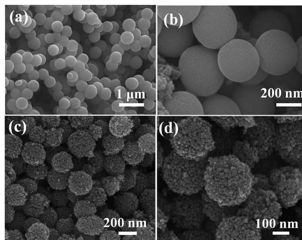
Fig. 2 FE-SEM images of TiO<sub>2</sub> colloids (a), (b), and TiO<sub>2</sub> beads (c), (d).
