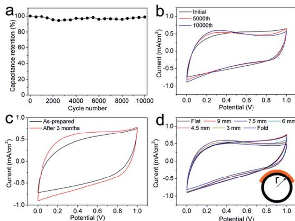
Fig. 5 (a) Cycling stability at a scan rate of 50 mV s<sup>-1</sup>, (b) CV curves of the initial, 5000th, and 10 000th cycles, (c) CV curves of the as-prepared C/TiO<sub>2</sub> MSC and the MSC after 3 months (scan rate 50 mV s<sup>-1</sup>), and (d) CV curves of MSCs bent with different curvature radii (scan rate 50 mV s<sup>-1</sup>). Inset in (d) is a schematic picture of a single MSC bent at different curvature radii.
