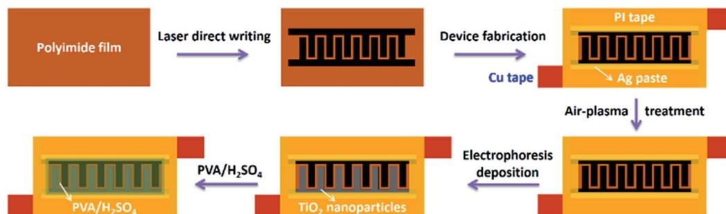
Fig. 1 Schematic illustration for the fabrication of a carbon/TiO<sub>2</sub> micro-supercapacitor with photo-rechargeable capability.
