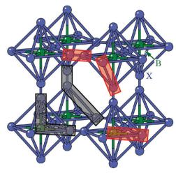
Representation of the simplified molecular perovskite structure used in our lattice-dynamical model. B atoms (shown in green) are located at the origin of the Pm3m cell, and X atoms (shown in blue) are located on the 6e site. The network is held together by a combination of harmonic bond stretching potentials (relevant pairs highlighted in red) and bond angle potentials (relevant triplets highlighted in black).
