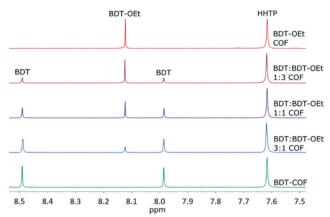
5 <sup>1</sup>H-NMR spectra of the hydrolyzed COFs showing stoichiometric incorporation of BDT and BDT-OEt linkers into the respective frameworks.
