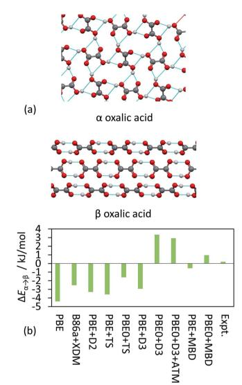
Fig. 4 (a) The hydrogen-bonding interaction in  $\alpha$  and  $\beta$  oxalic acid. (b) The relative energies between the polymorphs from experiment and as obtained with a number of different DFT methods.
