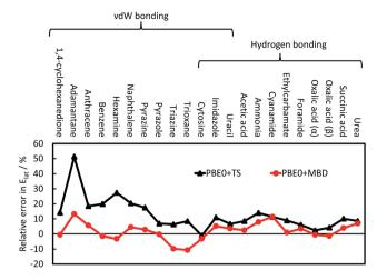
Fig. 3 The relative error in the calculate lattice energies for 22 vdWbound and hydrogen-bonded systems. A positive value indicates overestimation of the experimental lattice energies; see ref. 41 for more details and a discussion on CO2.
