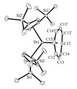
Fig. 4 Molecular structure of  $Cp_2^{\prime\prime}Th(C_8H_8)$ , 4. Thermal ellipsoids are drawn at the 50% probability level and hydrogen atoms are omitted for clarity.  $Th-C(C_8H_8)$  distances (Å): Th-C12, 2.815(4); Th-C13, 2.841(4); Th-C14, 2.769(3); Th-C15, 2.736(4).
