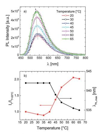
Fig. 3 (a) The effect of temperature on the fluorescence characteristics of P-2 in PBS (0.1 g  $L^{-1}$ ). The excitation wavelength was 435 nm. (b) The correlation between  $\lambda_{\text{max}}^{\text{PL}}$ , the relative emission intensity  $(I_T/I_{T=20 \text{ °C}})$ , and the temperature of the solution. Data are taken from the spectra in (a).
