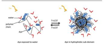
**Scheme 1** Idealized mechanism of fluorescence sensing in aqueous media through the coil-to-globule transition of a thermoresponsive polymer. As long as the (solvatochromic) fluorophore is exposed to water, the fluorescence intensity is weak. When heated above the LCST, the fluorophores get embedded in less polar and less fluidic sub-domains formed of collapsed chains, and emit more strongly at a blue-shifted maximum.
