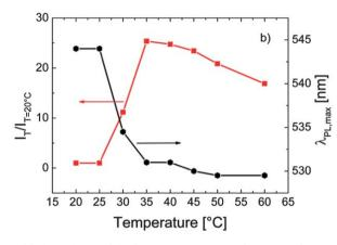
**Fig. 2** (a) The evolution of the fluorescence spectrum of **P-1** in PBS (0.1 g L $^{-1}$ ) with temperature, recorded at an excitation wavelength of 450 nm. (b) The correlation between  $\lambda_{\rm max}^{\rm PL}$  the relative emission intensity  $\langle l_7/l_{7=20}$  °c), and the temperature of the solution. Data are taken from the spectra in (a).
