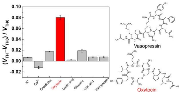
**Fig. 3.** Result of the selectivity test against eight types of chemical species (*i.e.*, D-glucose (10 µg/mL), creatine (0.3 µg/mL), L-lactic acid (18 µg/mL), uric acid (8 µg/mL), potassium ion (K<sup>+</sup>) (547 µg/mL), calcium ion (Ca<sup>2+</sup>) (48 µg/mL), vasopressin (10 pg/mL), and oxytocin
