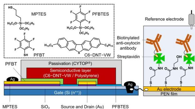
**Fig. 1.** Schematic illustration of the extended-gate-type OFET sensor for oxytocin detection.
