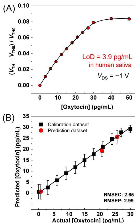
**Fig. 4.** (A) Titration isotherm of the oxytocin detection in human saliva at pH = 7.5. [Oxytocin] = 0–50 pg/mL. The errors at 0–50 pg/mL were 2–12 %. (B) Spike recovery test for oxytocin using human saliva.
