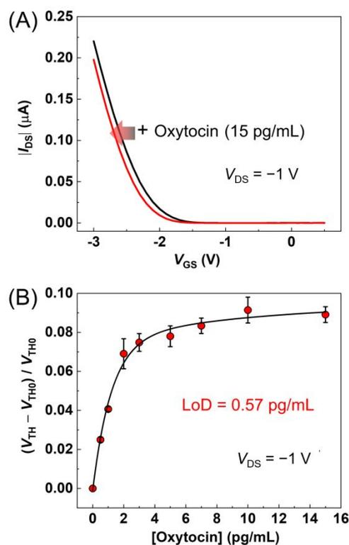
**Fig. 2.** (A) Transfer characteristics of the biotinylated anti-oxytocin antibody modified OFET upon the addition of oxytocin in D-PBS buffer solution containing Tween 20 (0.05wt%) and human serum albumin (0.1wt%). (B) Titration isotherm of the oxytocin detection. [Oxytocin] = 0–15 pg/mL. The errors at 0–15 pg/mL were 3–12 %.
