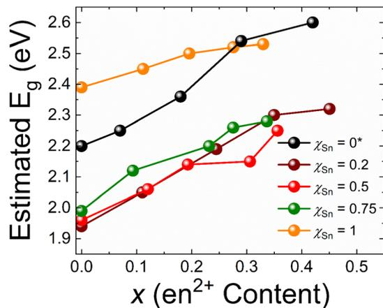
Fig. 10 Depicts the trend in estimated  $E_g$  (eV) as a function of the experimentally determined ethylenediammonium content. \*The  $\chi_{\text{Sn}} = 0$  line is plotted based on data from our previous works.<sup>38</sup>
