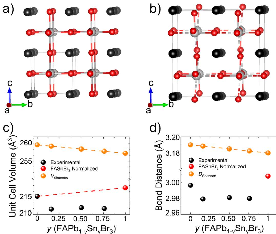
Fig. 5 (a) The overall structure for FAPb<sub>0.5</sub>Sn<sub>0.5</sub>Br<sub>3</sub> and (b) FASnBr<sub>3</sub> as displayed down the crystallographic a-axis, (c) the trend in the experimental unit cell volume compared to the theoretical Shannon volume as a function of Sn content, and (d) the trend in bond distance compared to the predicted Shannon distance as a function of Sn content. The atoms are shown in grey, silver, red, and black for Pb, Sn, Br, and FA<sup>+</sup> respectively.
