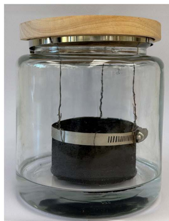
Fig. 1 Schematic and image of the experimental set-up for the static surface (core) leaching procedure (SSLP).
