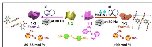
Fig. 14 Effect of milling conditions on the 1-1 + 3-3 disulfide exchange in the presence of DBU. Under NG conditions (left), the reaction yields mostly Form A of 1-3 (80–85 mol%), with 15–20 mol% unreacted 1-1 and 3-3 . Under LAG conditions (right), Form B of 1-3 is obtained quantitatively. 41,53
