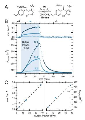
Fig. 5 (A) Equilibrium between  $10Me_{tBu}$  and OT. (B) Mole fraction of the Z isomer and overall system  $K_{eq}$  ( $K_{eq,sys}$ ) of  $10Me_{tBu}$  equilibrated with OT during the NMR photoisomerization experiment at varying LED output powers (3.2 to 37.6 mW). (C) Mole fraction of Z isomer and maximum system  $K_{eq}$  versus LED output power.
