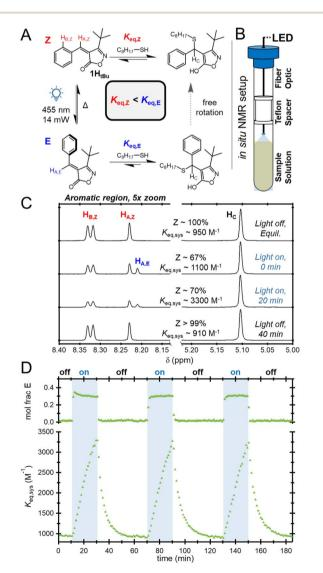
Fig. 3 (A) Equilibria involved in thiol-bonding and photoisomerization. (B) Diagram of the in situ LED NMR setup. (C)  $^{1}$ H NMR spectra of  $1H_{tBu}$ equilibrated with OT without and during irradiation with 455 nm light. (D) Cycling experiment (455 nm irradiation for 20 min followed by a 40 min dark interval) for 1H<sub>tBu</sub> equilibrated with OT.
