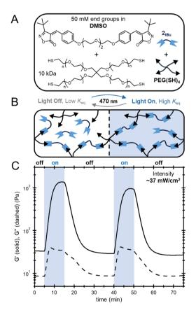
Fig. 7 (A) Chemical structures used in the synthesis of the organogel. (B) Diagram demonstrating increase in thiol-bonding and network connectivity upon irradiation. (C) Storage and loss moduli of the organogel during cycles of irradiation (470 nm) and darkness.
