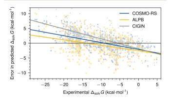
Fig. 7 Error in computed solvation energy ( $\Delta_{solv}G$ ) versus experimental  $\Delta_{solv}G$  for three representative models: COSMO-RS (QM, blue circles), ALPB (SQM, yellow squares), and CIGIN (ML, gray triangles). Solid lines show linear regression lines of the errors, indicating each model's systematic underestimation of large (positive) and overestimation of small (negative) values. All values are given in kcal  $mol^{-1}$
