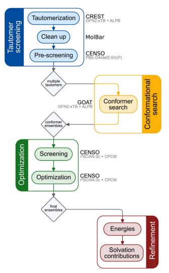
Fig. 3 Illustration of the workflow used to generate the structure ensemble for a given substance in a given phase. The used software/ tool (black) and level of theory (gray) is given as text next to the individual steps
